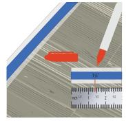
3. On a new section from the tape roll, make a mark 1-3/8" from end as shown.
