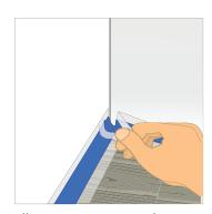
5. Pull tape corner out as shown and press the upper adhesive strip straight into the corner.
