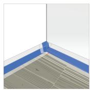
7. When tape strip is flat against wall, press and seal the upper adhesive strip.
